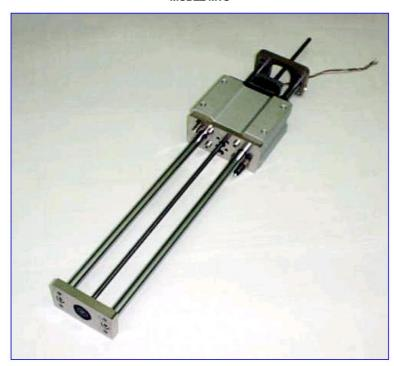
The thruster slide is a stepper motor driven lead screw slide. The body of the Thruster is mounted to your frame or to another slide. The tooling plate telescopes out and away from the slide base to any programmable position within the maximum stroke of the slide. Thruster slides can hold position when power is removed, and can be mounted in any orientation.
